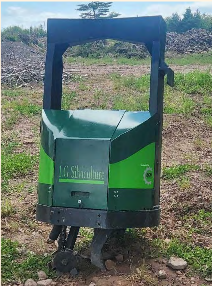
The prototype mechanical seeder, ready to be attached to a harvester.
